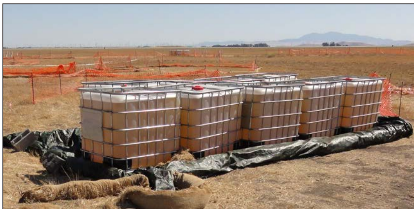
Supersized Salad Dressing: Plastic totes such as these are used to transport and store large quantities of emulsified vegetable oil (EVO). EVO injections into a body of solvent-contaminated groundwater has proven to be an effective groundwater cleanup method at Travis AFB. (Photograph by Glenn Anderson)
