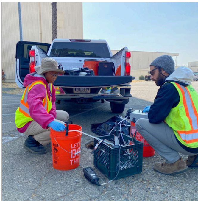
Contractor Siting: Two field specialists collect water samples that will be analyzed in a laboratory for PFAS constituents. Although this work appears to be routine, it is critical for maintaining high quality control standards and ensuring the most precise data. (Photograph by Megan Duley [Oneida])
