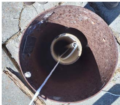
Typical Groundwater Monitoring Well at Travis AFB Photograph by Diane Escobedo, Oneida Team
