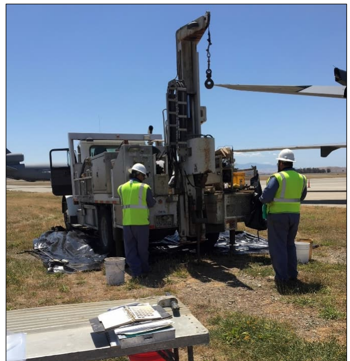
Photo 2: Direct-push drilling at Site SD031 in 2020. Photo Credit: Jacobs
