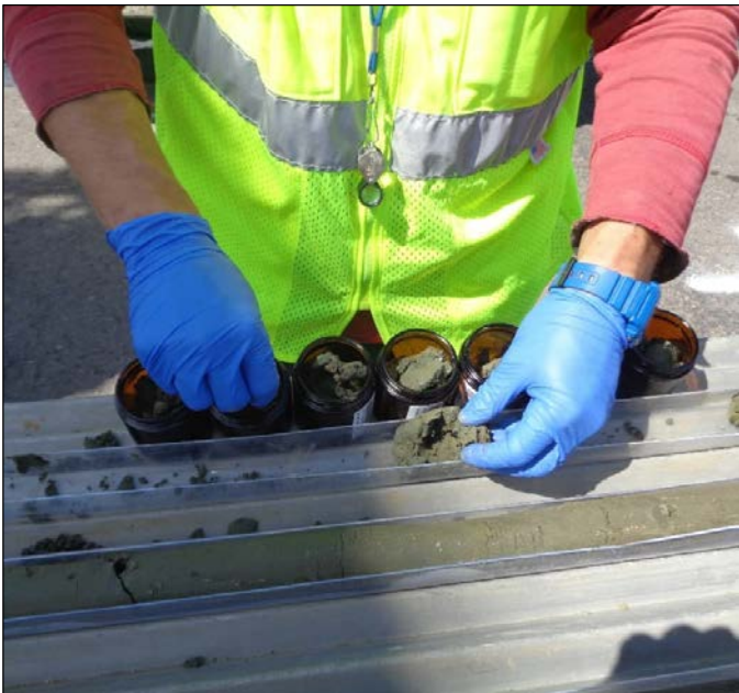
Photo 4: Collecting soil samples from a soil core in 2016. Photo Credit: Jacobs
