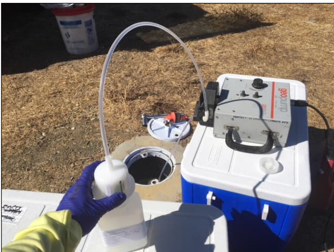
Photo 5: Collecting a groundwater sample from a newly installed monitoring well in 2020. Photo Credit: Jacobs
