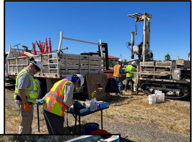
Oneida Team drilling and sampling soil
