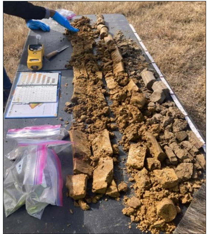
The Oneida project geologist logs soil collected in acetate liners from borings during Field Event #2. The soils are logged to capture data on soil types and characteristics to evaluate how constituents may interact or move in the subsurface environment.
