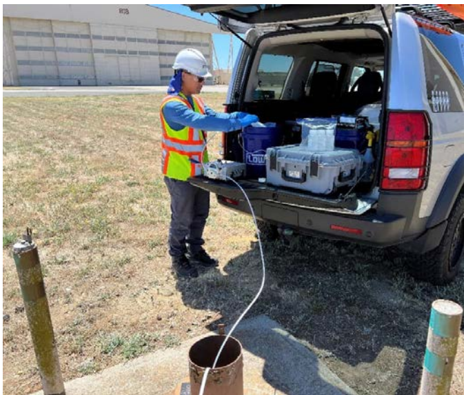
A field team member collecting a groundwater sample for PFAS analysis. Photo Credit: Oneida
