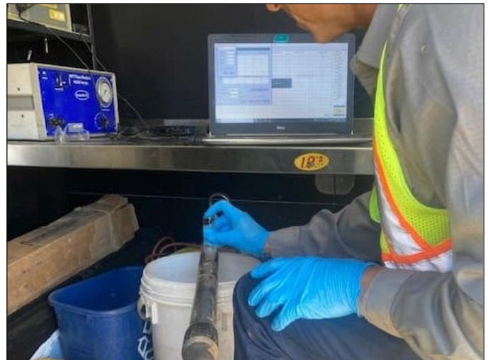
Figure 4. Technician performing a chemical response test on the MIP sensor. Photo Credit: Jacobs
