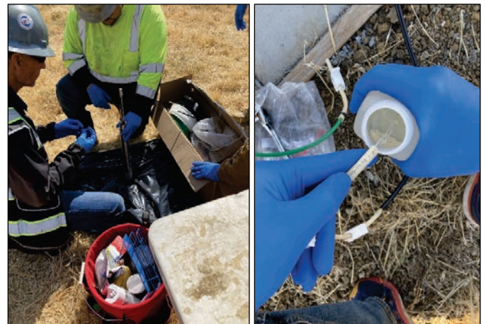
On the left, field staff prepare the stainless-steel lysimeter for installation. On the right, pore water is sampled during the October 2023 event. (Photo credit: Oneida)
