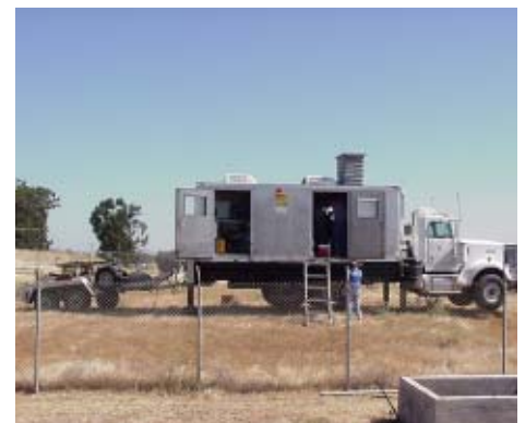
A Site Characterization and Analysis Penetrometer System collects water data at the base battery and electric shop, using specialized chemical sensors.
