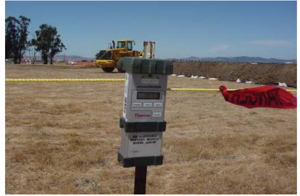
Dust monitoring equipment at several locations along the work area perimeter measures airborne contaminant concentrations.
