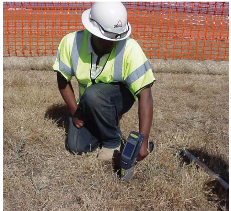
A field technician uses a portable XRF device to measure lead concentration in the surface soil at a former small arms range. Large numbers of detections in a short time period can guide decision-making in the field.
