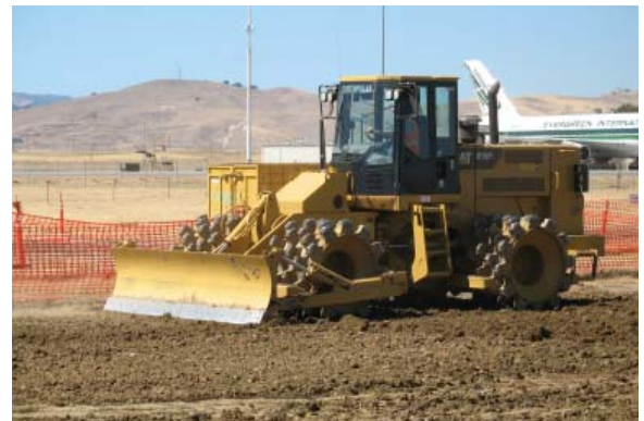
A sheeps-foot compactor moves backfilled soil across a cleaned site and compacts it to prevent future subsidence of the new soil.
