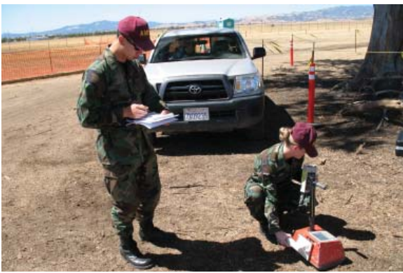
Members of the Travis AFB Radiation Safety Office conduct radiation checks on the outer casing of a nuclear density gauge.
