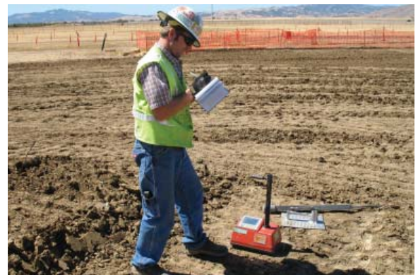
A field technician uses a nuclear density gauge to verify that the density of backfilled soil meets compaction requirements.
