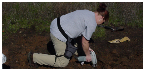
Ms. Jana Tarver from Oak Ridge National Laboratory measures the lead content in the soil at a former small arms range.
