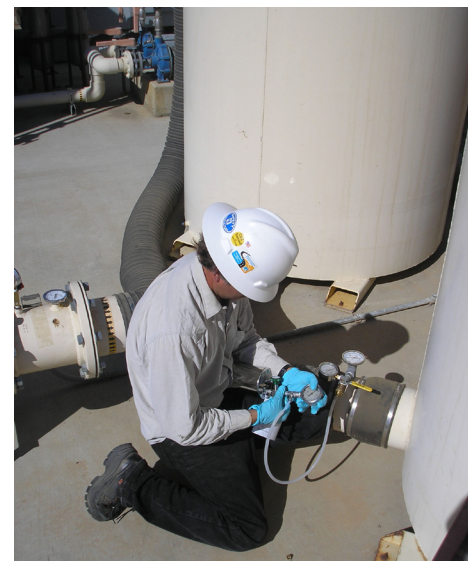
Mr. Rob Pexton from CH2M HILL collects a vapor sample between two carbon canisters, using a Summa air sample container.
