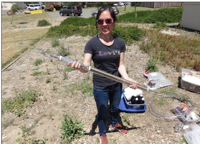
**Tool Time:** Sherry Peng, a UC Davis postdoctoral scholar, prepares the ISPT device for placement in a monitoring well downgradient from the Travis AFB gas stations. [Photo by Glenn Anderson]
