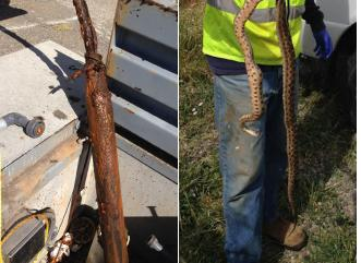
**Fieldwork Follies:** Suspended sediment in groundwater can coat an extraction pump (shown on the left), causing excess wear and tear and often leading to early pump failure. When field technicians discover the mechanical problems and visit the site to conduct repairs, they are often greeted by the local inhabitants, such as the non-poisonous snake shown in the right photo. [Photos by Eric Phelps (CH2M HILL)]
