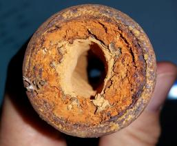
**Cleanup Coronary:** Groundwater pumps can change the chemistry of extracted water, bringing dissolved chemicals out of solution and resulting in the clogging of transfer piping. When the flow of water through piping is restricted, the treatment system's efficiency drops. [Photo by Doug Berwick (CH2M HILL)]
