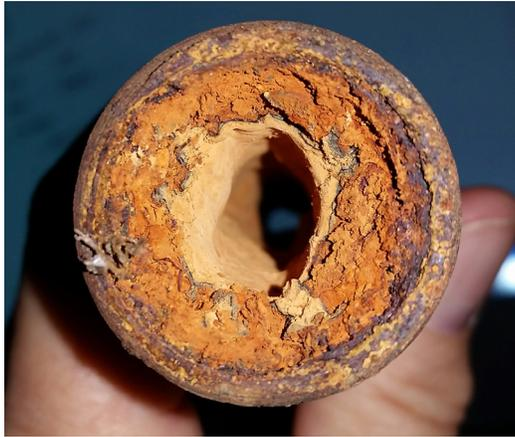
**Cleanup Coronary:** Groundwater pumps can change the chemistry of extracted water, bringing dissolved chemicals out of solution and resulting in the clogging of transfer piping. When the flow of water through piping is restricted, the treatment system’s efficiency drops. [Photo by Doug Berwick (CH2M HILL)]
