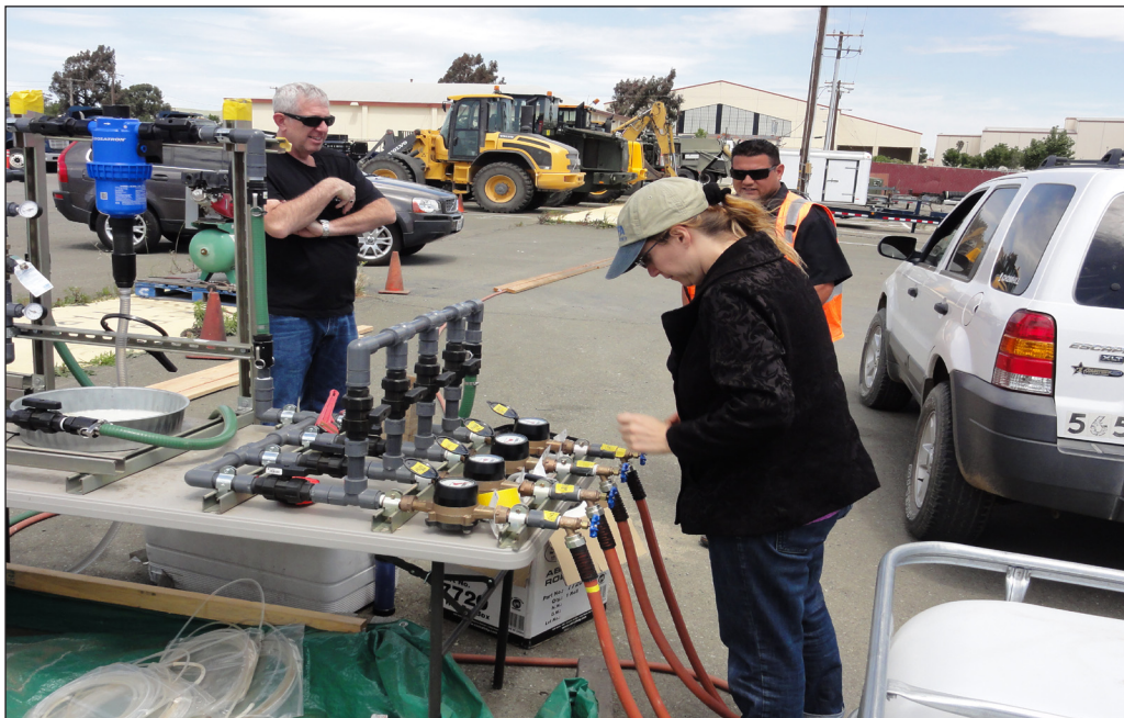
Going with the Flow: Ms. Nadia Burke from the U.S. Environmental Protection Agency checks the flow of vegetable oil that is injected into multiple wells at a solvent-contaminated groundwater site. Microbes in the groundwater consume the oil, triggering the breakdown of the solvents.
