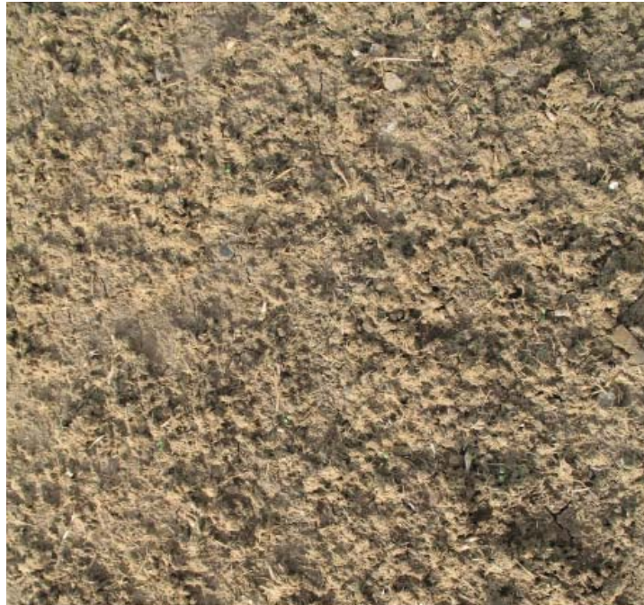
A Need for Seed: Individual seeds can be seen in this closeup of a hydroseed mixture on a soil surface. Pulp-like materials in the mixture serve to stabilize the soil and absorb water, promoting seed germination.
