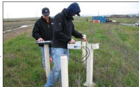
Environmental engineers take vapor readings from a network of soil gas monitoring wells surrounding the CAMU to check for the presence of methane.
