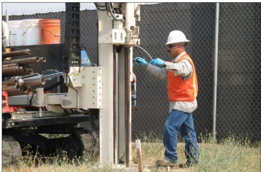
**Pushing Probes:** A field technician from Geoprobe, Inc. prepares to push a gas probe into the soil above groundwater that is contaminated with solvents. The plastic tube that protrudes from the top of the probe will be used to collect soil gas samples as part of a vapor intrusion assessment.
