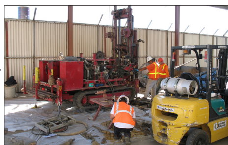
A field crew uses a track-mounted drill rig to collect soil borings within a building. This specialized rig is small enough to operate in confined spaces and powerful enough to collect samples from several hundred feet below the ground surface.
