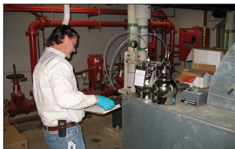
A laboratory technician from the Environmental Protection Agency sets up air sampling equipment in the mechanical room of an office facility. Air sample analysis will identify any solvent vapors that may enter from contaminated water beneath the building.
