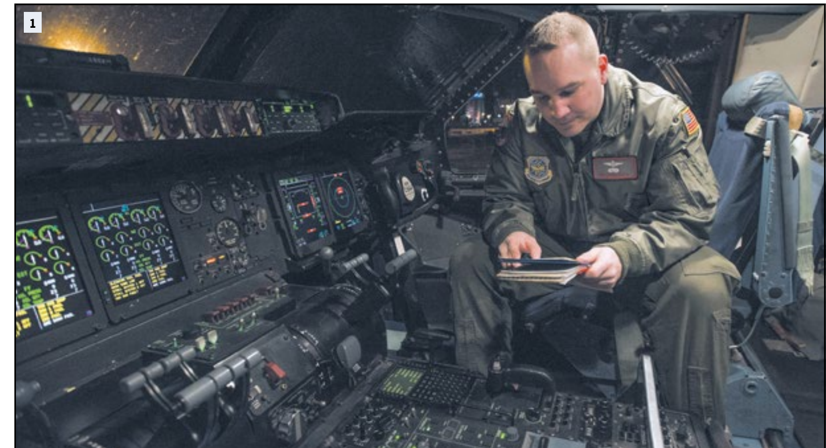
1) Tech Sgt. Timothy McCarthy, 22nd Airlift Squadron, completes a preflight inspection of the flight controls March 7 on a C-5M Super Galaxy at Yokota Air Base, Japan. As a flight engineer, McCarthy is responsible for completing preflight inspections of the aircraft prior to the pilots coming on board to ensure everything is safe for the flight.
