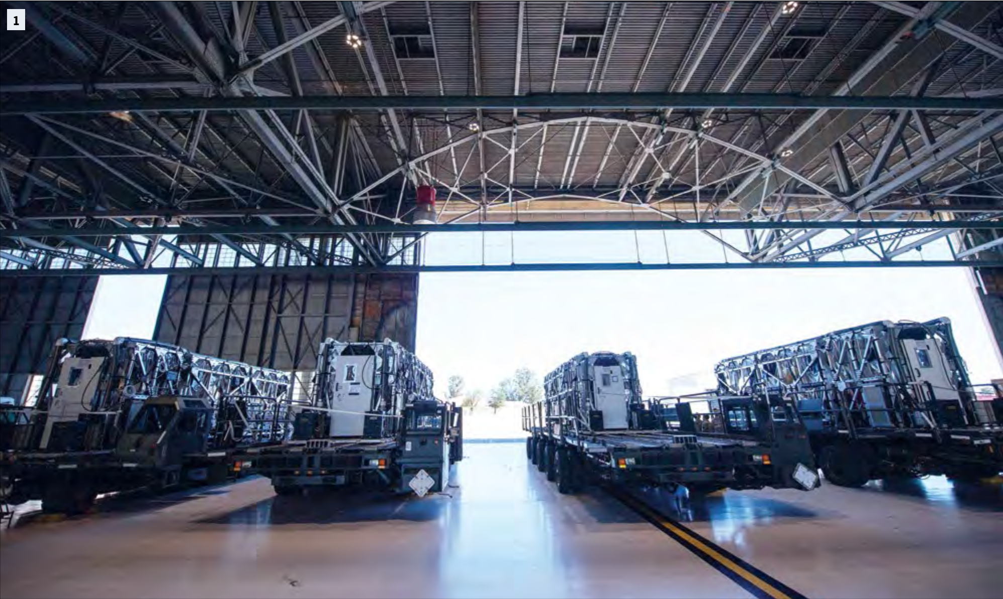
U.S. Air Force photos/Senior Airman Christian Conrad 1) Transport Isolation System capsules are positioned on respective cargo K loaders in a hangar April 28 at Travis Air Force Base, California. TIS capsules, which were initially engineered in response to the Ebola virus in 2014, allow the transport of individuals with highly contagious diseases without infecting any other passengers or aircrew on the aircraft. 2) U.S. Air Force Staff Sgt. Maranda Trujillo, 21st Airlift Squadron instructor loadmaster, boards a C-17 Globemaster III April 27 at Travis. 3) A C-17 is parked on the flight line April 27 at Travis. 4) U.S. Air Force Capt. Freddy Roman-Otero, 43rd Aeromedical Evacuation Squadron flight nurse, checks his equipment as part of a pre-flight procedure April 27 at Travis, California. Roman-Otero is one of two 43rd AES representatives called to perform training on the Transport Isolation System capsule. 5) U.S. Air Force Chief Master Sgt. Jennifer Moses, 775th Expeditionary Aeromedical Evacuation Flight, COVID West AE Task Force member, examines two Transport Isolation System capsules April 28 at Travis. 6) U.S. Air Force Capt. Steven Woods, 43rd AES Detachment 1 flight nurse, participates in a pre-flight meeting with other 43rd AES members April 27 aboard a C-17 at Travis.
